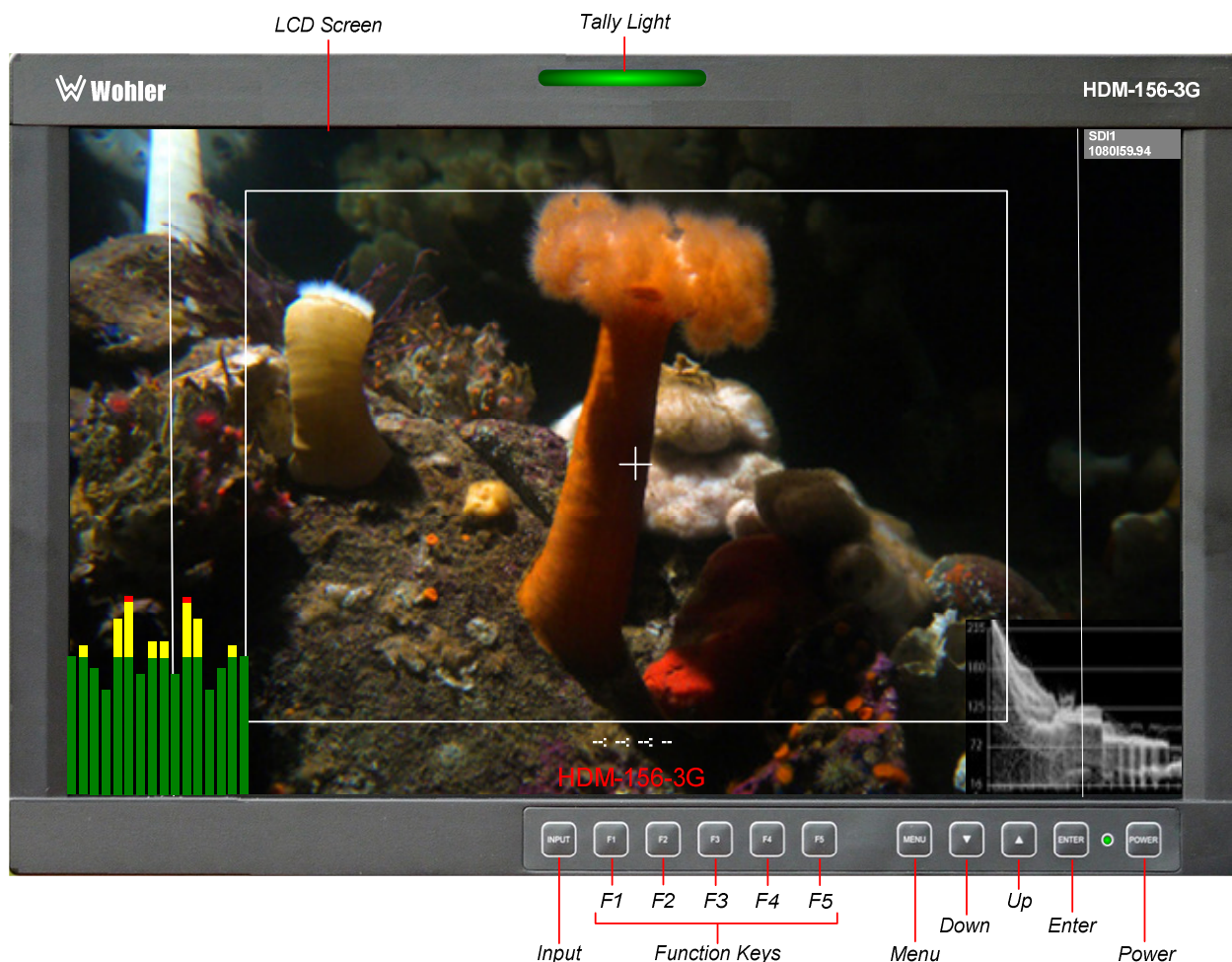
Figure 2–1: Front Panel Layout
