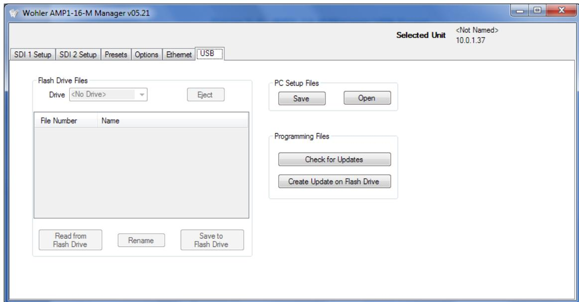
1. **Flash Drive Files:** This pane displays a list that shows the seven possible files in the **\Wohler** folder of the flash drive. If no **\Wohler** folder exists, the system will immediately create it when the flash drive is first connected. Clicking on any one of the files (or the empty file positions) selects it for other operations.
