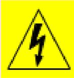
The symbol to the left warns of electric shock hazard inside the unit. Disconnect the power cord before removing access panels when installing upgrades. Only qualified service personnel are to operate the equipment with covers removed, and are to exercise caution to avoid personal injury.
