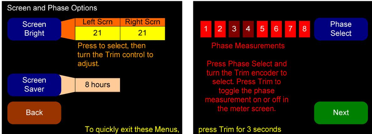
1. **Screen Bright:** Press this control to toggle between the adjustment for the left screen and the right screen. When a screen is selected, rotate the **Trim** knob to adjust the screen brightness. Thirty-two adjustment steps are provided for each screen from very dim to bright. The actual brightness of each screen will change as the control is turned. The default brightness for both screens is 21.
