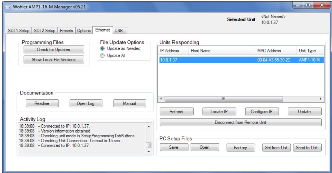
10. Once the unit appears, select it and complete any desired operations as described elsewhere in this manual. If the unit fails to appear after a few minutes, double check your connections and the instructions above about disabling unused Ethernet ports.
