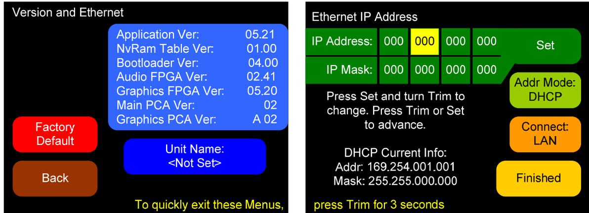
1. **Factory Default:** Pressing this button opens a cautionary window to verify that you really want to restore the AMP1-16-M setup to the factory default. If you press the **Factory Default** button again, the action proceeds and the unit will restart. Otherwise, after five seconds, the factory default request is cancelled. You can also cancel the factory default request by pressing any other button.
