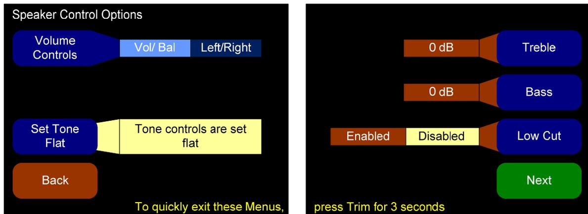
1. **Volume Controls:** You can use this option to change the master volume and the balance knob to become **Left Volume** and **Right Volume** controls.
