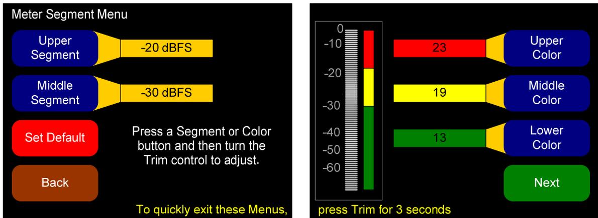
1. **Upper Segment:** Pressing this button and then rotating the **Trim** knob adjusts the division between the upper and middle segments. You can adjust the color boundary in 1 dB increments, and it has the same range as the bottom and top limits of the meter.
