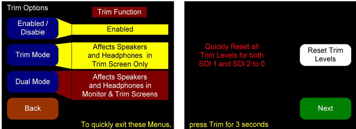
1. **Enable/Disable:** Pressing this button toggles the **Trim** feature on (enabled) and off (disabled). When disabled, pressing the **Trim** control will not enter the **Trim Screen**. Also, the **Trim** mode and **Dual** mode buttons are dark, but not disabled.
