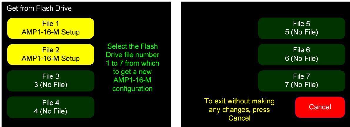
2. Using one of the bright yellow choices, press the file number (**File 1** through **File 7**) of the file you want to copy from your flash drive. When the copy process completes, the **Flash Drive Options** screen re-displays.
