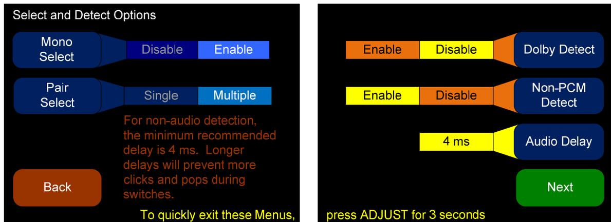
1. **Mono Select:** This control determines whether the **Channel Pair Select** buttons on the **Main Screen** can also select single channels, in addition to channel pairs.
