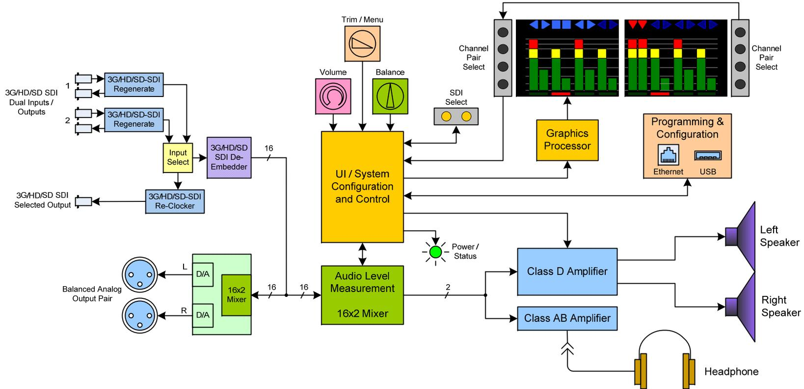
**Note:** Stereo phase indication measurement occurs in the signal chain before it is routed to the speakers.
