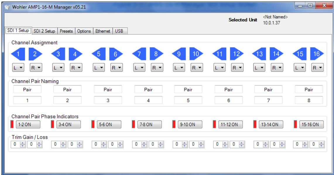
2. **Channel Assignment:** Click the drop downs to select whether each channel should be directed to the right, left, or both speakers.
