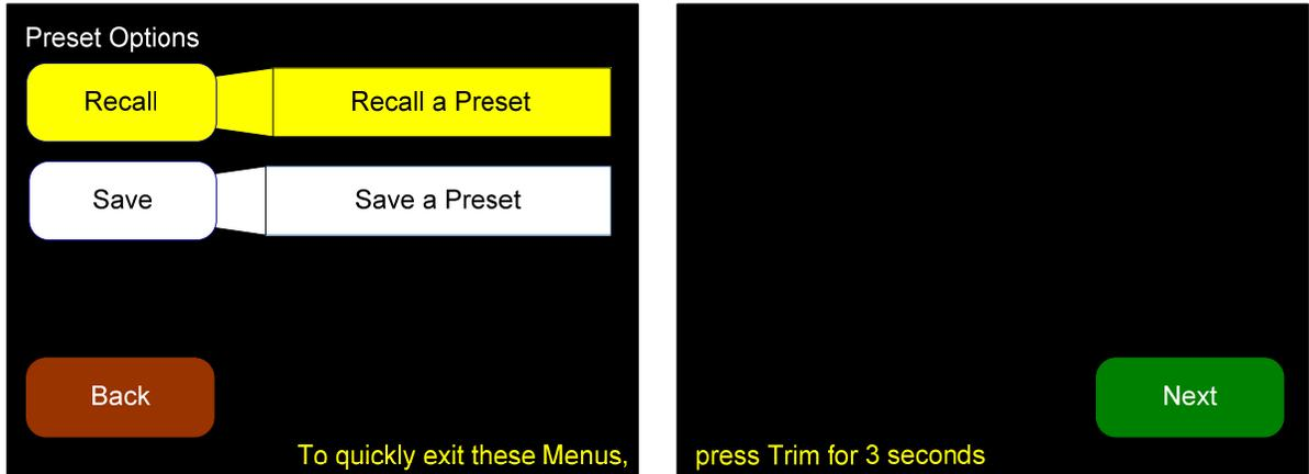
1. **Recall:** Pressing this button proceeds to the **Recall a Preset** screen as shown in Figure 4-4:
