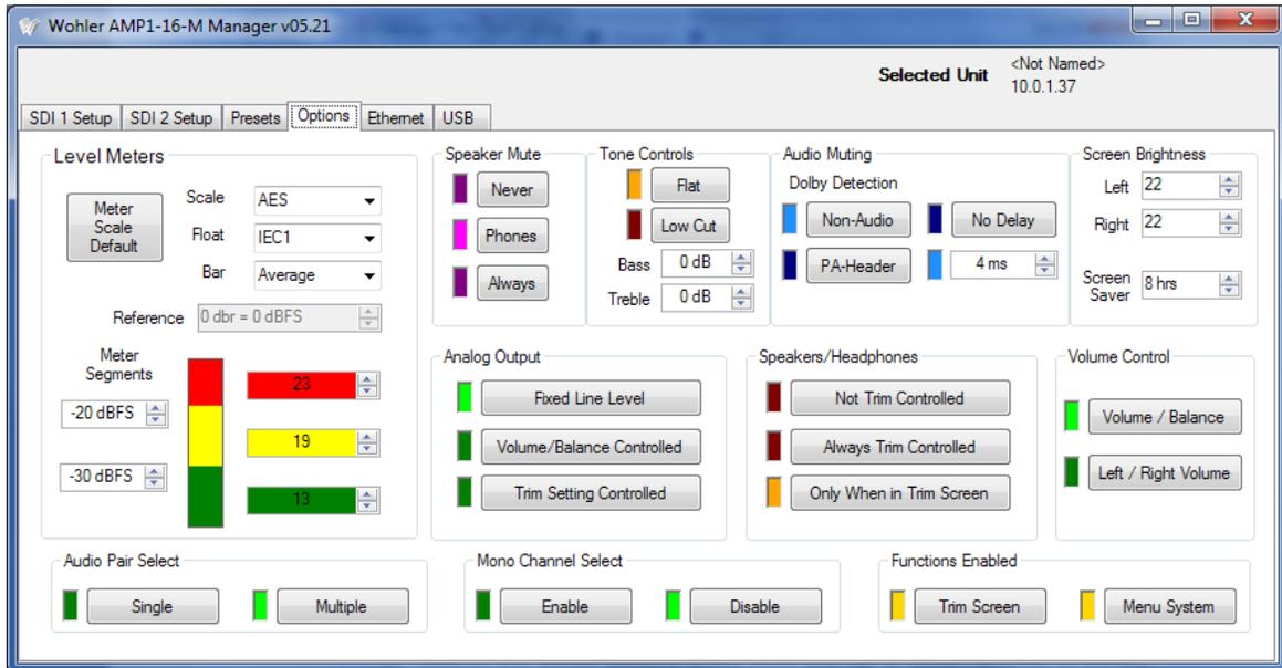
2. In the **Level Meters** area, click the drop downs to select **the Scale, Float, and Bar** for your level meter display. Alternatively, you can click the **Meter Scale Default** button to return to the default for that scale. The scale itself won't change.
