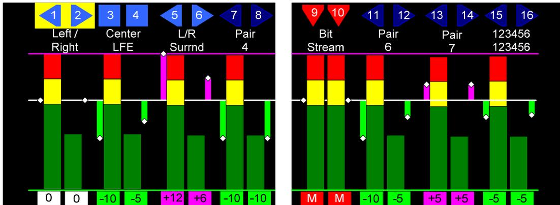
The meters are labeled as they are in the **Main Screen**. At the bottom of each meter, a number indicates the amount of gain or loss being applied to each channel. If a gain is being applied, the number is indicated in a pink square. If a loss is being applied, the number is indicated in a green square. If no gain or loss is being applied, a zero is indicated in a white square. Adjacent to each meter, a small graphical indication appears, showing the gain or loss from +12 dB to -40 dB.
