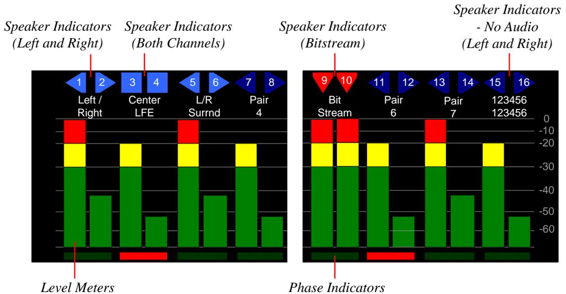
1. **Speaker Indicators:** The indicators above each meter identify the channel number and the status of the channel.
