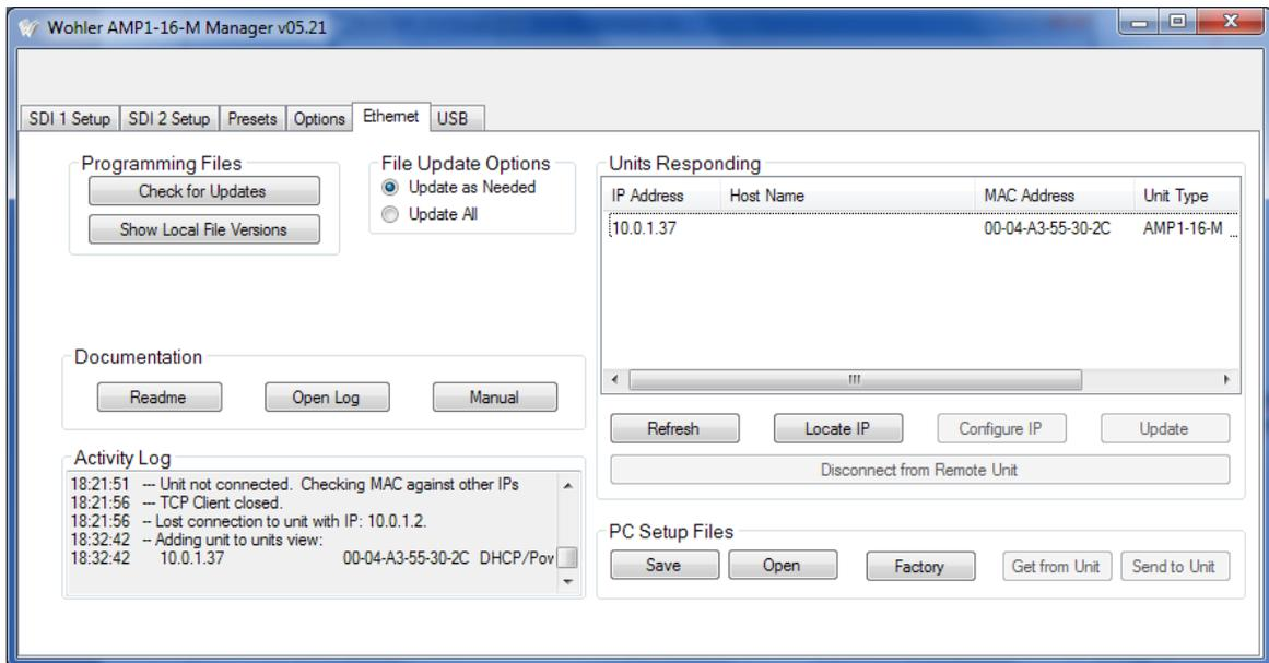
2. The **Ethernet** tab allows you to transmit configurations and perform a variety of other tasks over a network.
