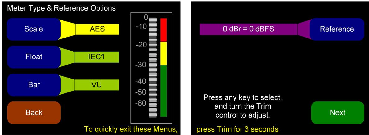
1. **Scale:** Pressing this button and then rotating the **Trim** knob steps through the scales for the level meters. Six selections are available as shown in [Table 4–1](#) below.
