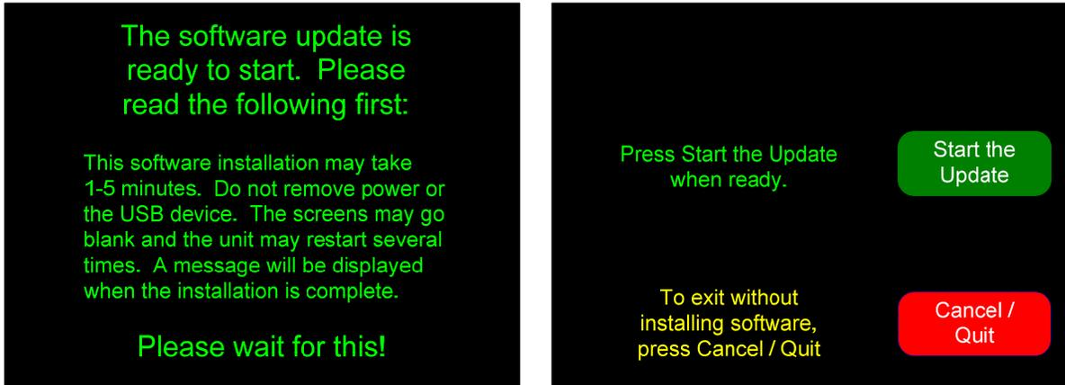
Read the advice on the screen so that you will know what to expect during the installation process. Pressing the **Start the Update** button will start the installation process, which will automatically continue until its conclusion.
