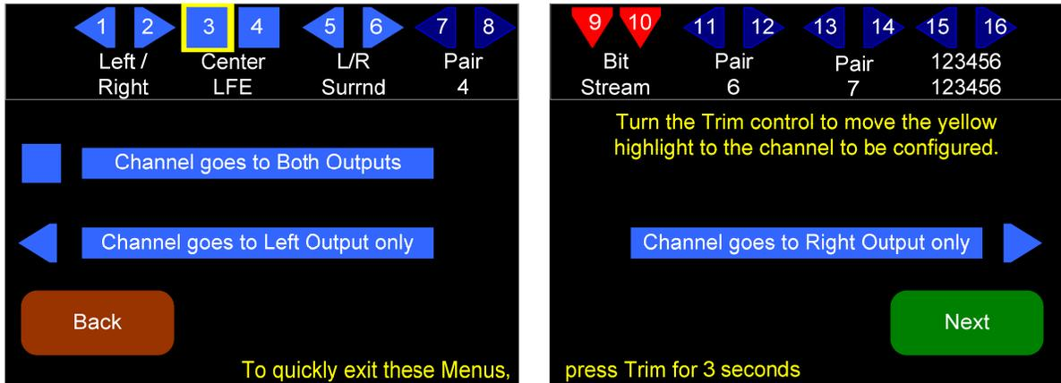
Turning the **Trim** knob left or right highlights each of the 16 channels in turn. Rotate to select a channel, then press **Channel goes to Both Outputs**, **Channel goes to Left Output only**, or **Channel goes to Right Output only**.
