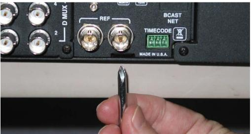
Figure 6–12: Remove Bottom Screw
