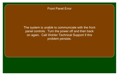
Figure 8-4: Front Panel Error Message
