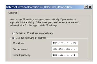
After making an IP address change such as this, close the control panel and reboot the host computer to be sure the change takes effect.
