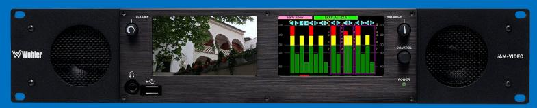
Intuitive monitoring and metering of video and audio from multiple sources, with touch screen controls, and APIs for remote management.
