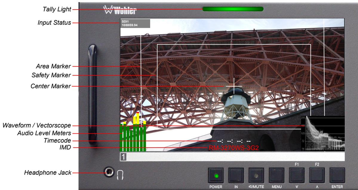
1. **Input Status:** Displays the selected input and video parameters of vertical active line count, (i)nterlaced or (p)rogressive, and field/frame rate in Hz.
