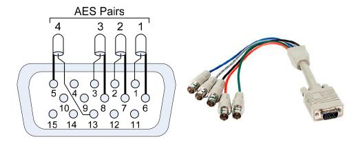
7. **AES Outputs**: This HD-15F connector provides 4 AES3id digital audio pairs (8 channels) at a 48 kHz sample rate from selected monitored sources. Refer to Figure 2-3 for the pinout of this connector. The easiest way to interface with this connector is to use an HD-15 to VGA adaptor cable. These outputs are <u>not</u> controlled by the **Volume** and **Balance**
