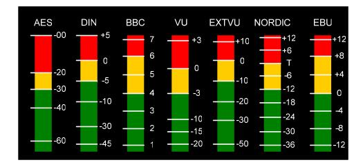
Figure 2-15: Meter Scale Selection
