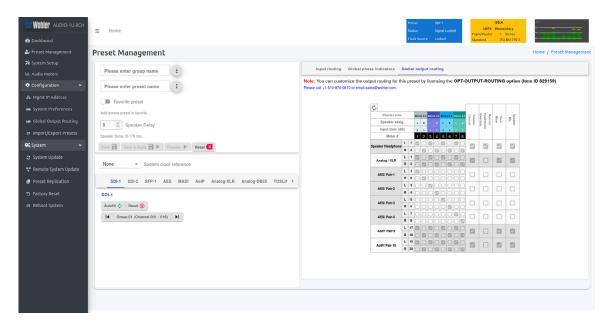
However, if the OPT-OUTPUT-ROUTING license is installed, this tab allows you to determine exactly which input channels are routed to which outputs. It then appears as shown in Figure 4-18. This very flexible capability allows you to route signals according to Preset or as a default for the whole system.
