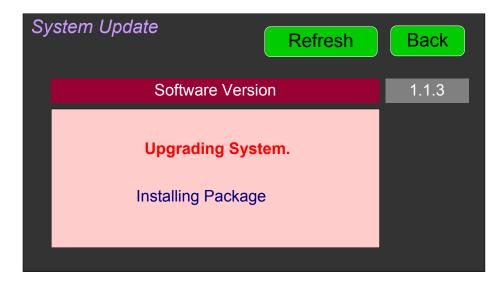
7. After the software update starts, the text on the left screen will change periodically to indicate the progression of the upgrade. The upgrade will take 5 minutes or more, after which the iAM2-8 will restart. After the system has completed its restart cycle and is once again operational, you may then remove the flash drive.
