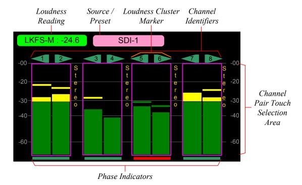
Figure 2-8: Audio Level Meter Screen
