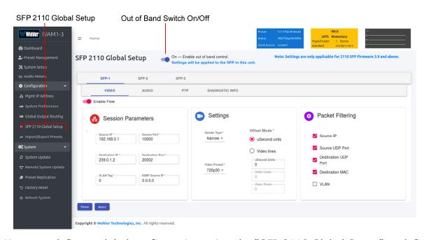
You may define a global configuration using the "SFP 2110 Global Setup" or define it on per Preset basis. Refer to the **SFP 2110 Preset Setup** section later in this Appendix. The global configuration will be used for Source Select. Refer Figures F-3 and F-4 for Video parameters. Refer to Figures F-5 and F-6 for Audio parameters. Refer to Figure F-7 for PTP parameters.
