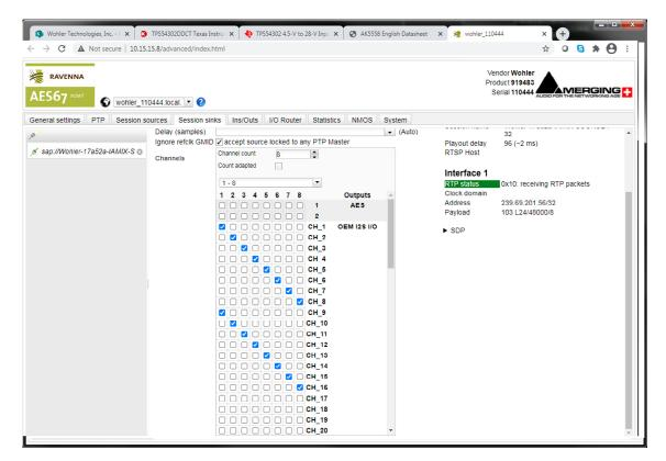
To avoid confusion if monitoring more than one Flow, especially if the various source Flows have overlapping channel numbers, use the matrix to direct Flows to higher channel ranges. For example, for monitoring 2 SDI sources (four 8 channel Flows), assign two flows to 1-8 and 9-16 and the next SDI signal to 17-24 and 25-32. Touch the iAM2-8 AOIP selection menu to select the proper range to monitor, up to 57-64.
