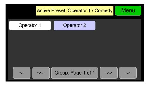
The Presets are normally arranged into Groups. Use this screen to select which Preset-containing Group to examine. After selecting one of the Groups, the Preset Selection screen shown in Figure 2-24 is shown.
