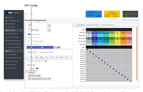
Figure F-8: SFP 2110 Preset SFP Configuration Enable
