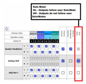
The setting shown above determines that outputs will follow the Audio Meter screen solos & mutes for the XLR outputs because the checkbox is checked. It is not checked for the AES outputs, so they will not be affected by the solo & mute choices. This feature requires the optional OPT-OUTPUT-ROUTING output routing license.
