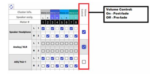
How do I make the XLR outputs follow the Audio Meter screen solos & mutes while the AES Pair-1 does not?
