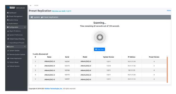
Figure 4-21: Preset Replication Scanning Screen
