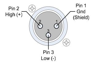
10. **Analog Outputs:** These male XLR connectors provide two balanced analog outputs: Left and Right. The source of these signals is the mix of audio as monitored by the internal speakers and is adjusted by the **Volume** and **Balance** controls. The **Analog Outputs** are standard on the iAM2-8. Refer to Figure 2-5 for the pinout of this connector.
