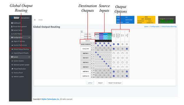
Figure 4-20: Global Output Routing Option
