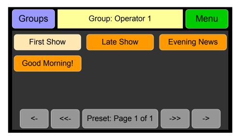
To select a Preset, touch the associated button. After a quick 2-second delay, the metering screen will display the channels contained in that source.
