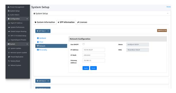
Figure F-1: SFP IP Address Configuration
