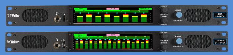
8 channel or 16 channel, baseband only, shallow depth, dual 3G-SDI inputs, AES3 & analog audio monitor with a 7" wide touchscreen.
