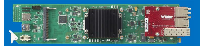
Wohler monitor in openGear form factor that ships standard with 12G SDI I/O and can be accessed via remote GUI in place of traditional front panel.
