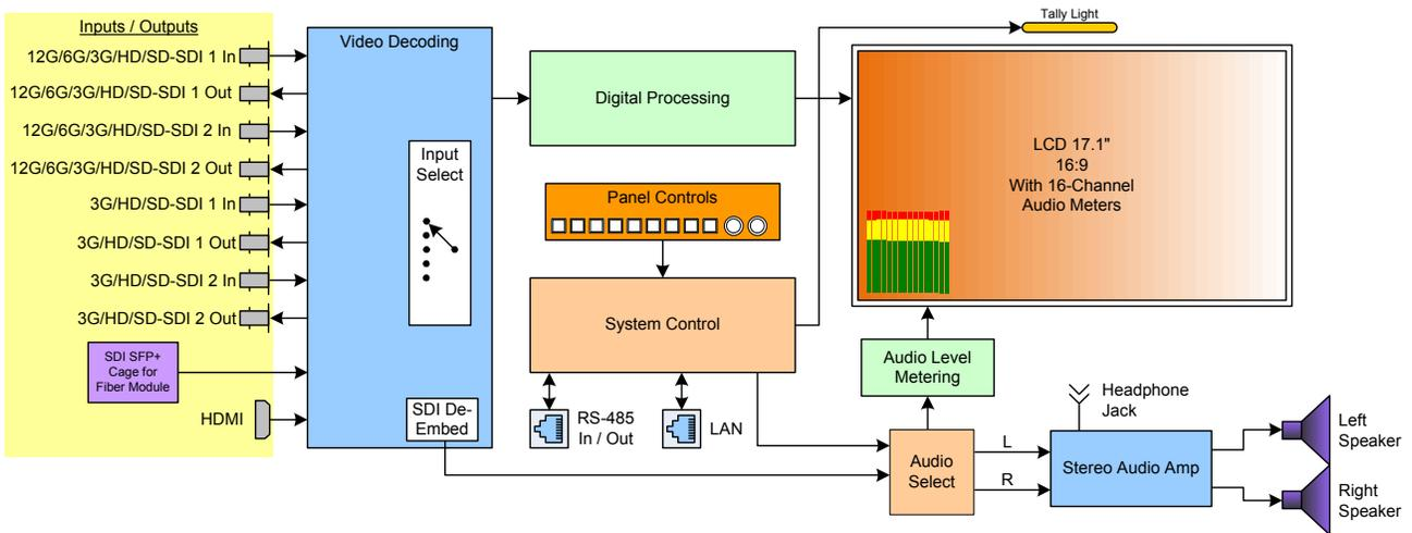
Figure 3-2: vMON-240-4K Block Diagram
