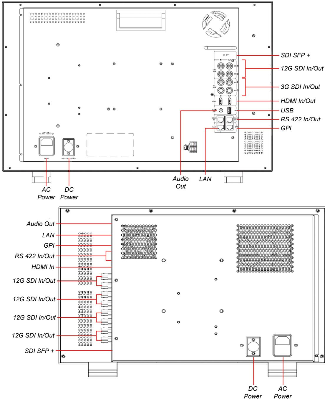
1. **AC Power:** The monitor receives power from the AC inlet, which is a standard IEC receptacle for 100 to 240 VAC  $\pm 10\%$ , 50/60 Hz power connection, and includes a Power Switch. Normally the Power switch is kept in the "1" (On) position and the operation of the monitor is controlled from the front panel controls. Four regional AC power cords, supplied according to shipping region, are available.
