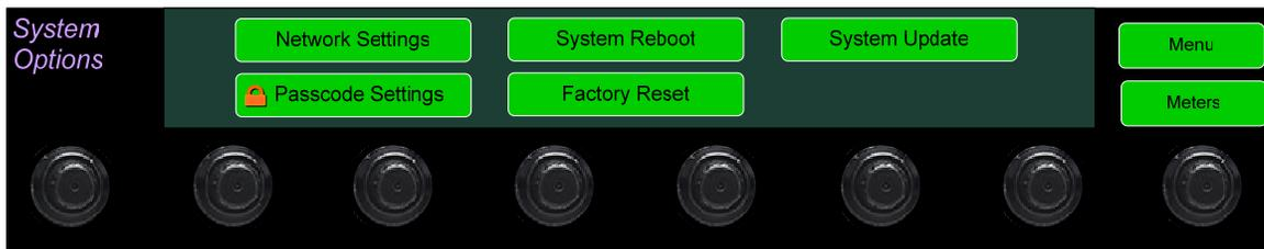
Touching the **Passcode Settings** selection in the **System Options** menu proceeds to the **Passcode Entry** screen as shown in Figure 2-30.
