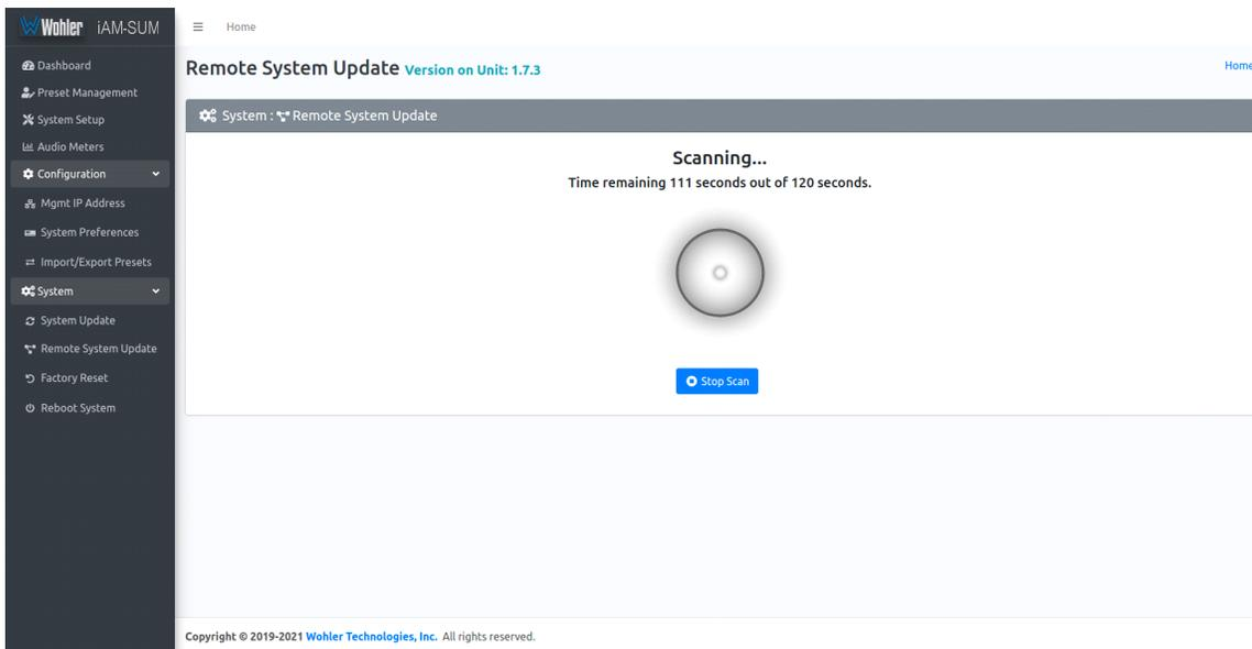
**Note:** The scanning process will take 2 minutes. Progress is shown on the screen. If for some reason you would like to stop the scan prematurely, click the **Stop Scan** button.
