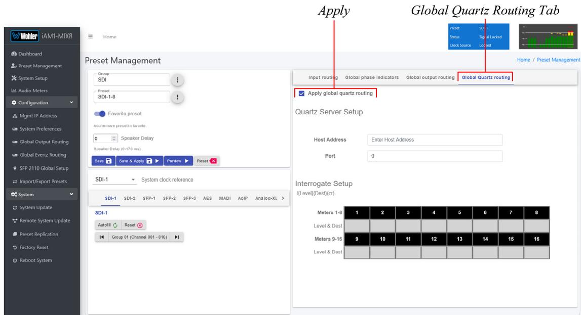
The Global Quartz Routing Tab will display the Quartz Server Setup and allow you to decide whether Global Quartz Routing will apply to this Preset.
