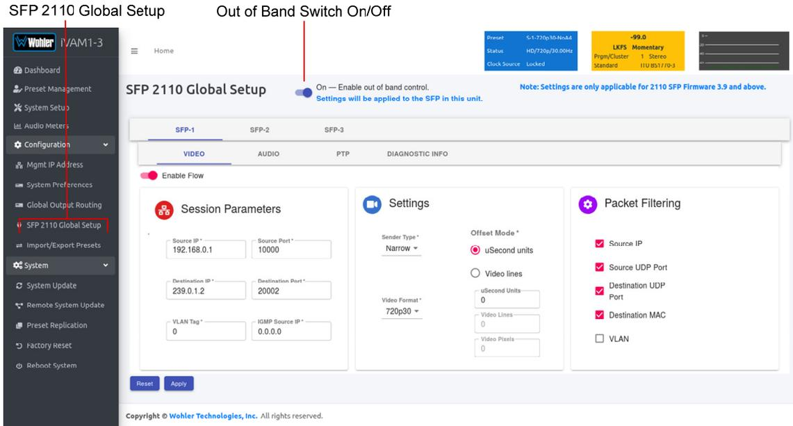
You may define a global configuration using the “SFP 2110 Global Setup” or define it on per Preset basis. Refer to the **SFP 2110 Preset Setup** section later in this Appendix. The global configuration will be used for Source Select. Refer Figures F-3 and F-4 for Video parameters. Refer to Figures F-5 and F-6 for Audio parameters. Refer to Figure F-7 for PTP parameters.
