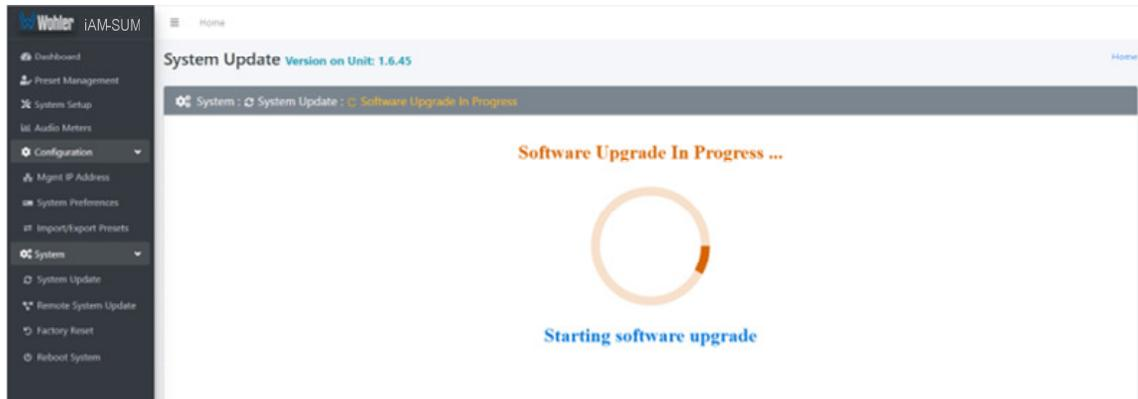
7. At this point, wait for the update to complete. It may take several minutes, but **it is critical not to disturb the iAM1-MIX8 or the Web GUI** until the update process is complete. When it is complete, the iAM1-MIX8 will restart.
