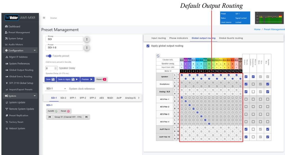
However, if the OPT-OUTPUT-ROUTING license is installed, this tab allows you to determine exactly which input channels are routed to which outputs. It then appears as shown in Figure 4-15. This very flexible capability allows you to route signals according to Preset or as a default for the whole system. Refer to the **Global Output Routing** section in this chapter to learn the function of each of the checkboxes and of the matrix in this tab.
