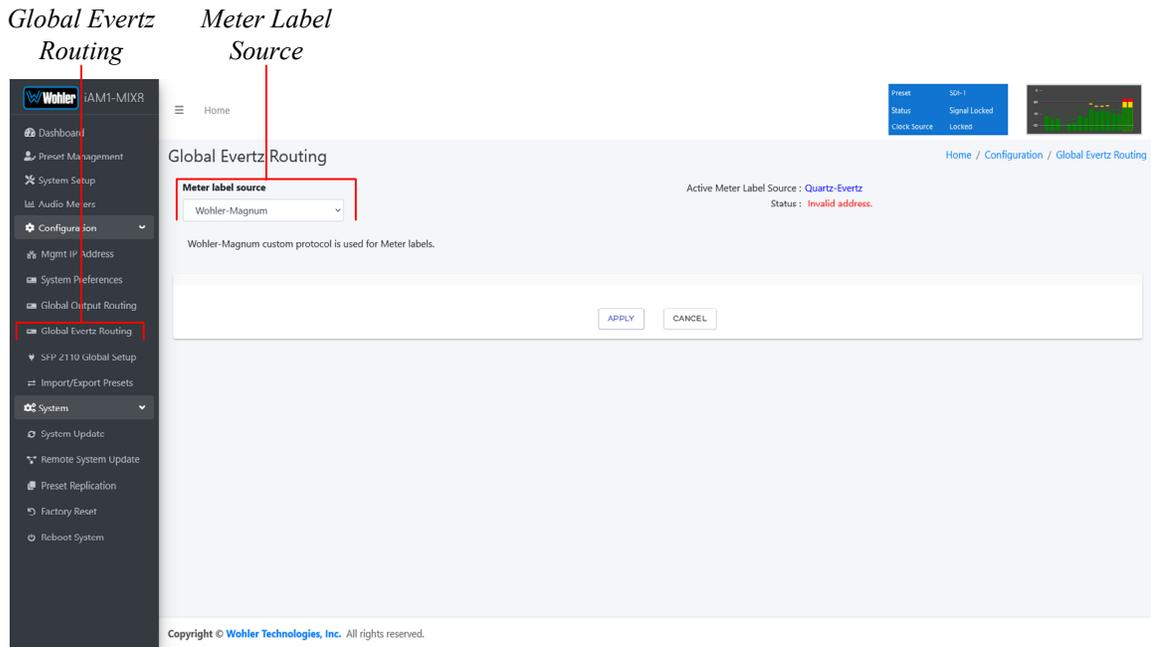
Set the Meter Label Source on this screen to “Evertz Quartz” as shown in the following figure:
