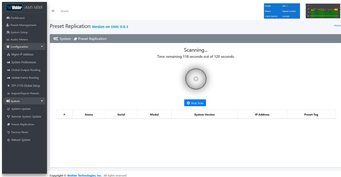
Once all the units are discovered you may either copy the presets that are currently created on the Master unit or can use an external preset file that you want to copy to any or all of the Target units. **Note that any and all of the Presets that may already be contained in each Target unit will be erased by copying the new Presets.**
