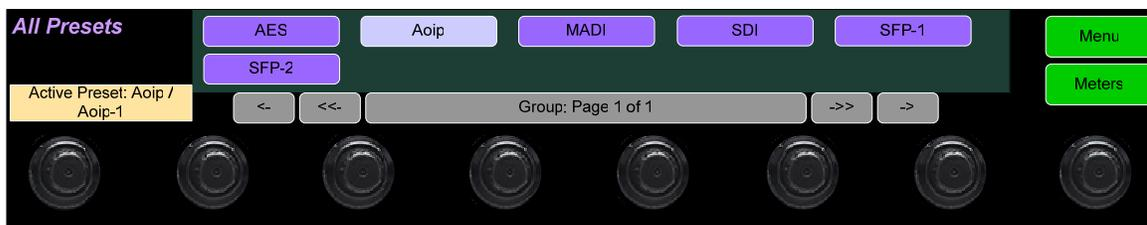
The Presets are normally arranged into Groups. Use this screen to select which Preset-containing Group to examine. After selecting one of the Groups, the Preset Selection screen shown in Figure 2-14 is shown.
