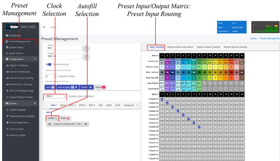
1. **Preset Configuration:** You may create a new Preset, adjust an existing Preset, or create a new Preset from an existing Preset:
