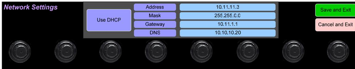
1. To change the IP Address, Net Mask, Gateway, or DNS, tap the item you would like to change. A keypad will appear, as shown in Figure 2-24.
