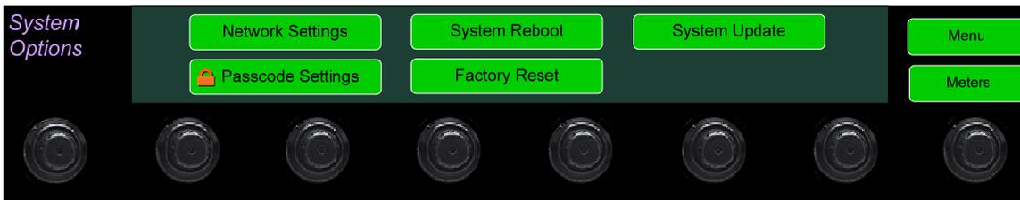
4. In the **System Options** menu, touch **System Update**. The **Software Upgrade** screen will appear, as shown in Figure A-2.
