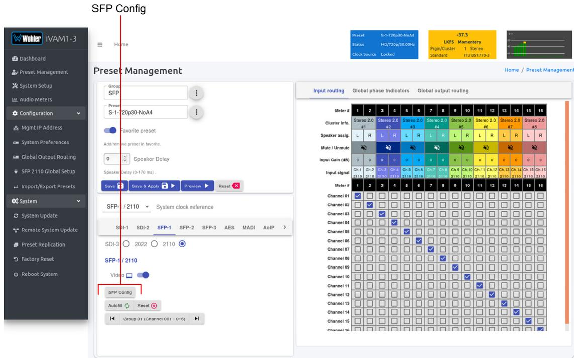
After clicking the **SFP Config** button, the **SFP 2110 Setup Screen** will appear, as shown in Figure F-9. Make the settings you need for this Preset and then click **Close**.
