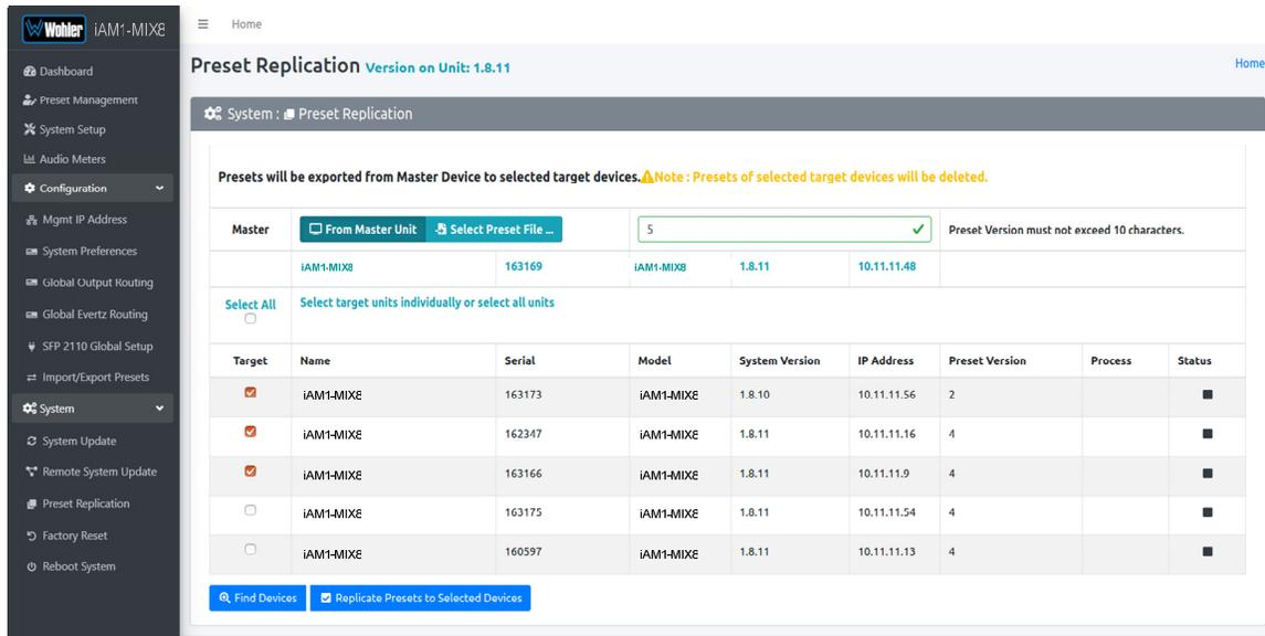
Click either **From Master Unit** or **Select Preset File**. This determines the source of the Presets to be copied. Preset Files would be files that you have previously stored in the computer running the Web GUI.
