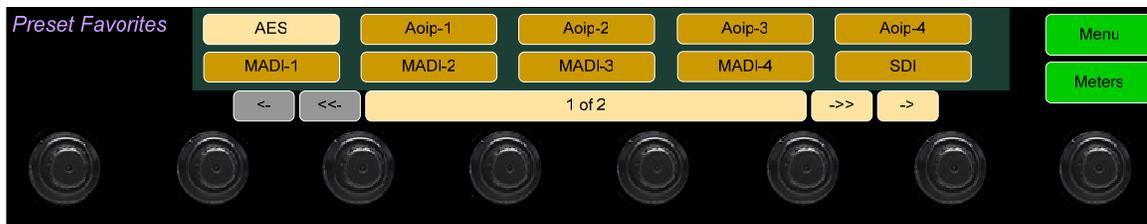
In this screen, the currently selected Preset is shown in bright yellow. Touch any Preset to select it or rotate the **Source/Presets** knob to navigate to your choice and then press it.
