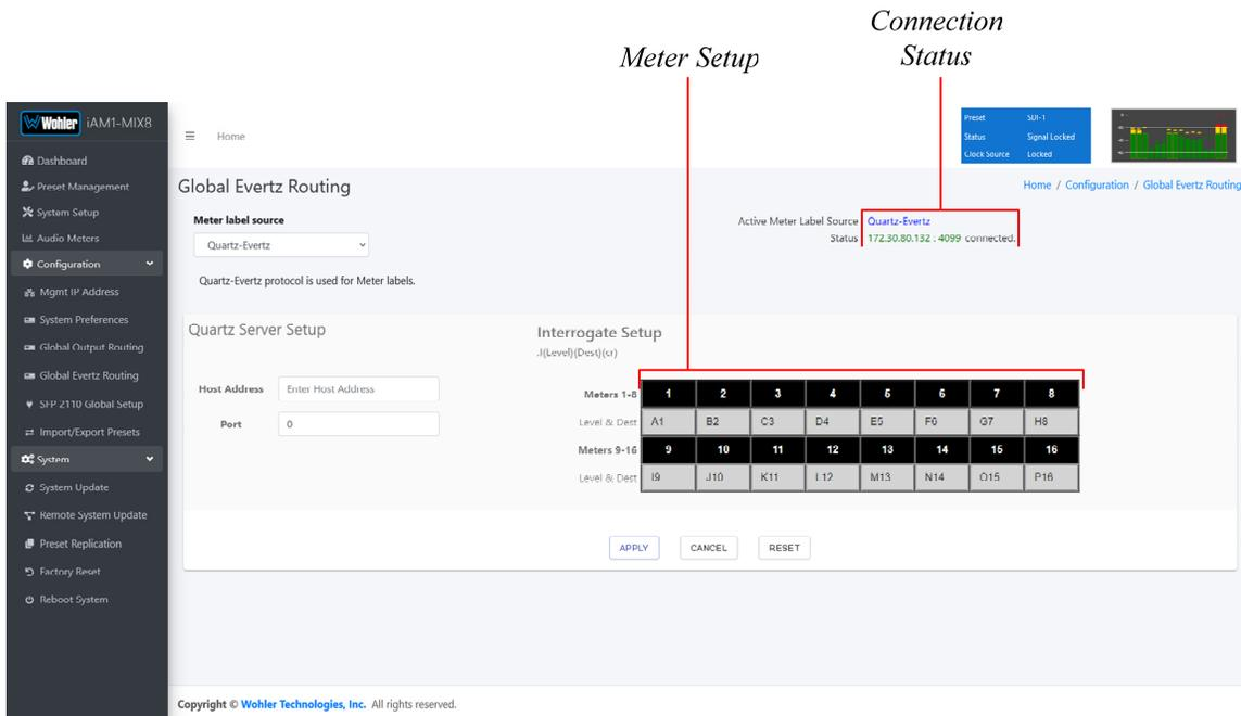
Verify that the Connection Status indicates that it is connected. The Interrogate Setup section will show the new meter label setup, now synchronized with the Evertz Quartz Server.
