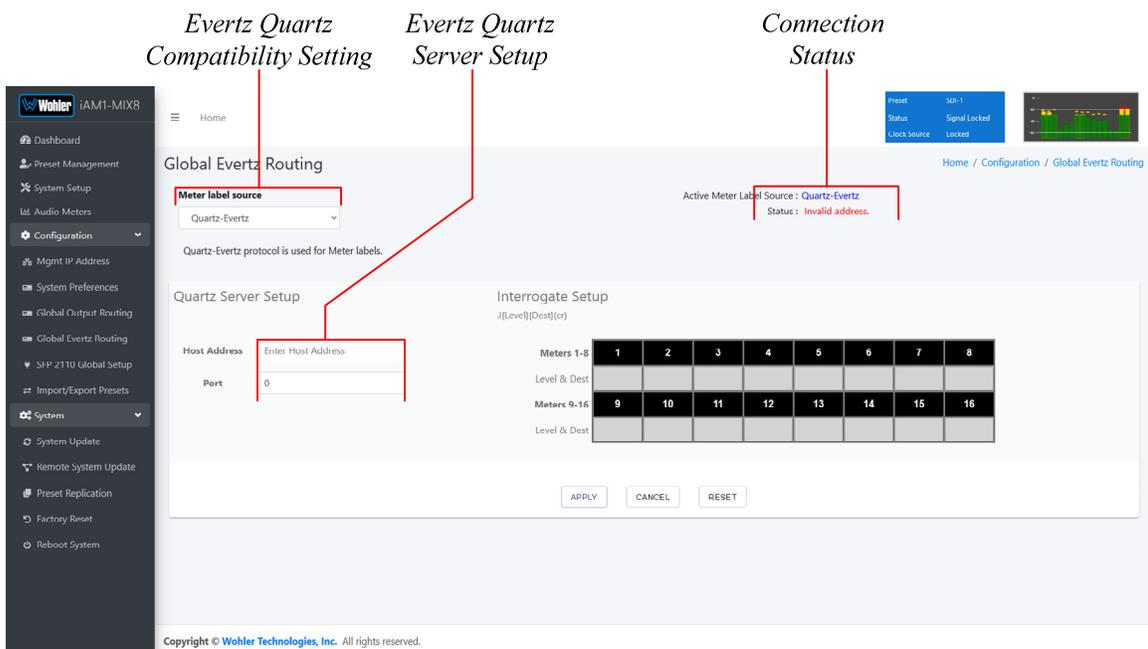
If no Evertz Quartz Server Setup is entered, or if it is incorrect, the Connection Status will indicate Invalid Address. Enter the Host Address and Port of the Evertz Quartz server in the Quartz Server Setup section. For assistance, contact Wohler Technical Service. Click the **Apply** button to enable Evertz Quartz compatibility. When Evertz Quartz compatibility is enabled and connected, this screen changes as shown in the following figure:
