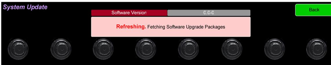
5. The new software version that is in the flash drive will be shown in the **Software Version** screen. To cancel the upgrade at this point for any reason, touch **Back**. To proceed, touch the software version entry in the **Software Version** screen. A screen will appear to verify you would like to perform the upgrade.
