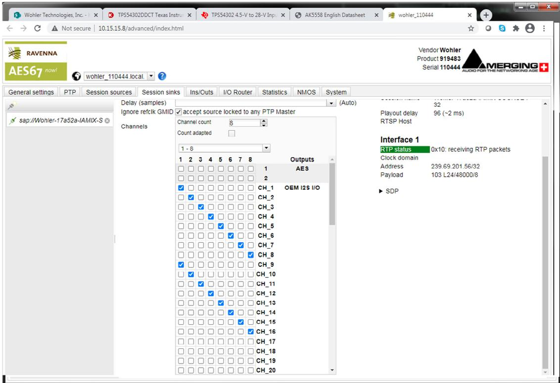
To avoid confusion if monitoring more than one Flow, especially if the various source Flows have overlapping channel numbers, use the matrix to direct Flows to higher channel ranges. For example, for monitoring 2 SDI sources (four 8 channel Flows), assign two flows to 1-8 and 9-16 and the next SDI signal to 17-24 and 25-32. Touch the *iAM1-MIX8* AOIP selection menu to select the proper range to monitor, up to 57-64.
