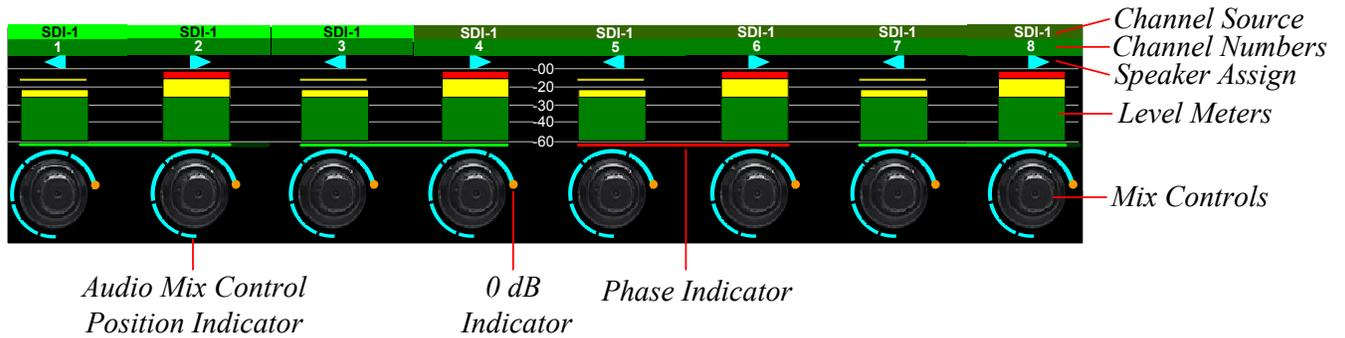
1. **Channel Source:** The name of the input source of each channel or channel pair is shown. If this designation is dark, the channel or channel pair is not included in the mix. However, if the block containing the name is bright green, then channel or channel pair is part of the mix. The text of the Channel Source may be set using the Web GUI. Refer to Chapter 4.
