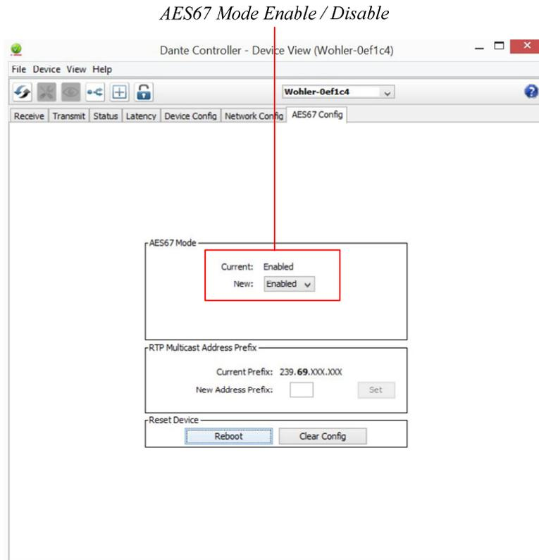
Further, Dante AES67 discovery and operational protocol requires manual assignments for static multicast transmit and receive IP addresses per Dante protocols for discovery and IGMP network operation. Destination addresses in range 239.nnn.0.0 – 239.nnn.255.255, port 5004 or nnn can be configured using the Dante Controller. The default is 69. The destination and receive address range must match. Provisions for this are in **Dante Controller Device View - Network Config**. Refer to Figure B-6.
