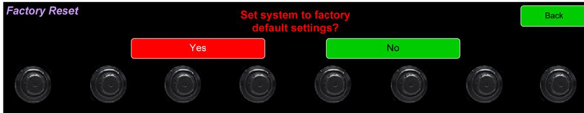
**Note: Factory Reset** will also reset your IP address to the default one. After a Factory Reset, the IP Settings will need to be updated. The default IP address for the unit is determined based upon the Mac address. It is 169.254.1.xx where xx is the last octet of the management Mac address. For example, if the Mac address is b4:ed:54:d0:04:28 then the IP address would be 169.254.1.40 (40 is the decimal equivalent for the last octet of Mac address 28.)
