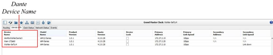
During initial setup, you may want to manually change the *iAM* unit **Name** in the [System Setup](#) page to match the reassigned **Dante Device Name** for consistency. Refer to Figure B-3.
