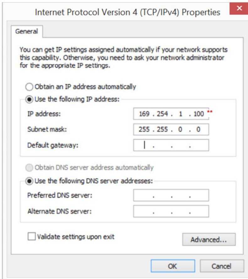
\*\* The actual IP address to enter here is located on the System IP Address line of the System Details screen.
