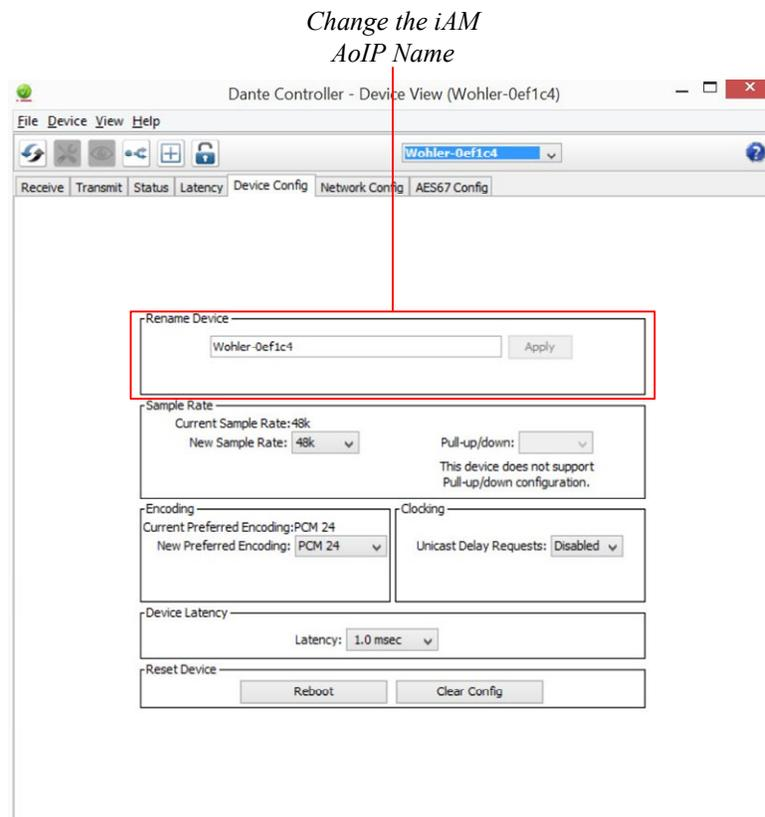
Other changes such as **Latency** settings can be made by the Dante Controller through the **Device View** menus. Some changes may require remote rebooting of the Brooklyn II card to take effect, temporarily interrupting audio and publishing the new information to the network.
