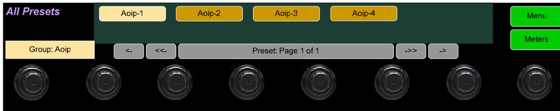
To select a Preset, touch your selection or rotate the **Source/Presets** knob to navigate to your choice and then press it. After a quick 2-second delay, the metering screen will display the channels contained in that source.
