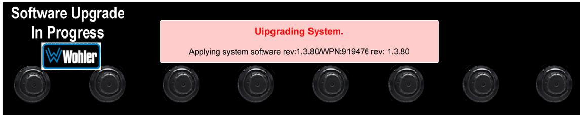
After the software update starts, the text on the screen will change periodically to indicate the progression of the upgrade. The upgrade will take 5 minutes or more, after which the *iAM1-MIX8* will restart. After the system has completed its restart cycle and is once again operational, you may then remove the flash drive.
