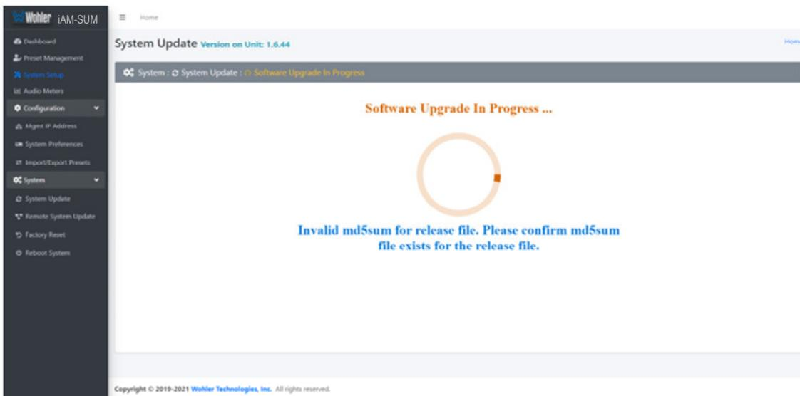
3. At this point, wait for the update to complete. It may take several minutes, but **it is critical not to disturb the iAM1-MIX8 or the Web GUI** until the update process is complete. When it is complete, the iAM1-MIX8 will restart.
