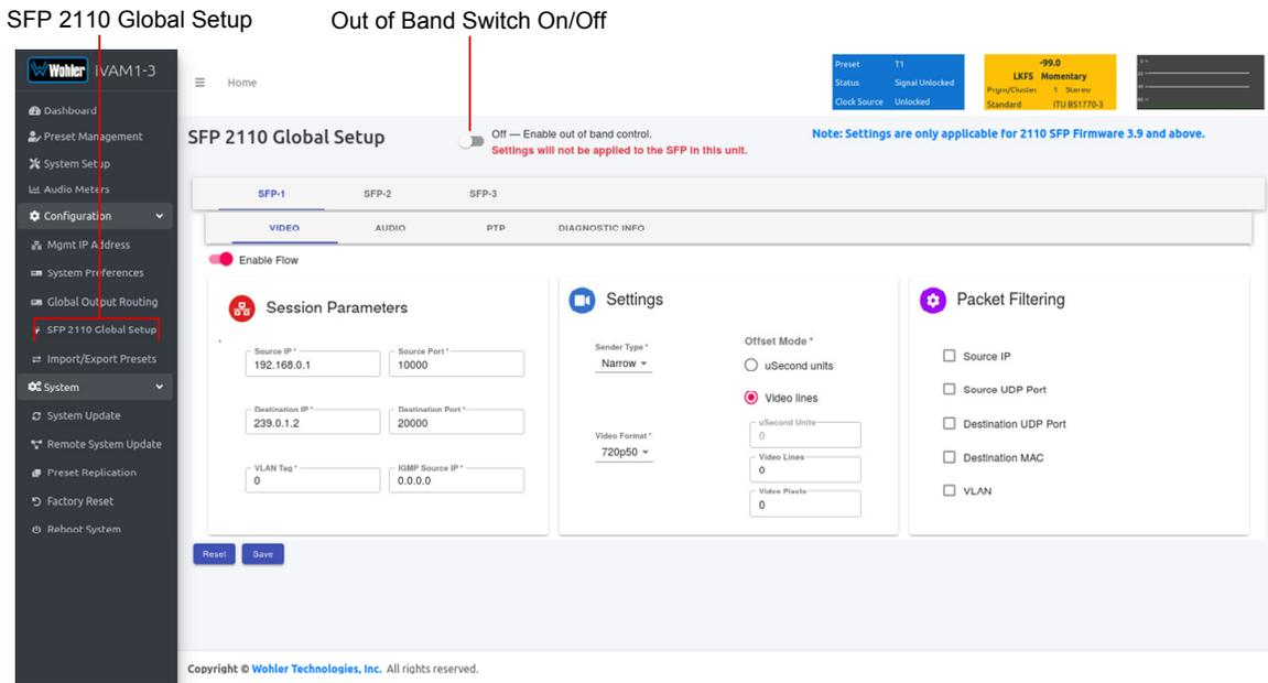
When the **Out of Band On/Off Switch** is turned **On**, as shown in Figure F-4, the Wohler monitor will internally communicate with the SFP to configure the flow information.
