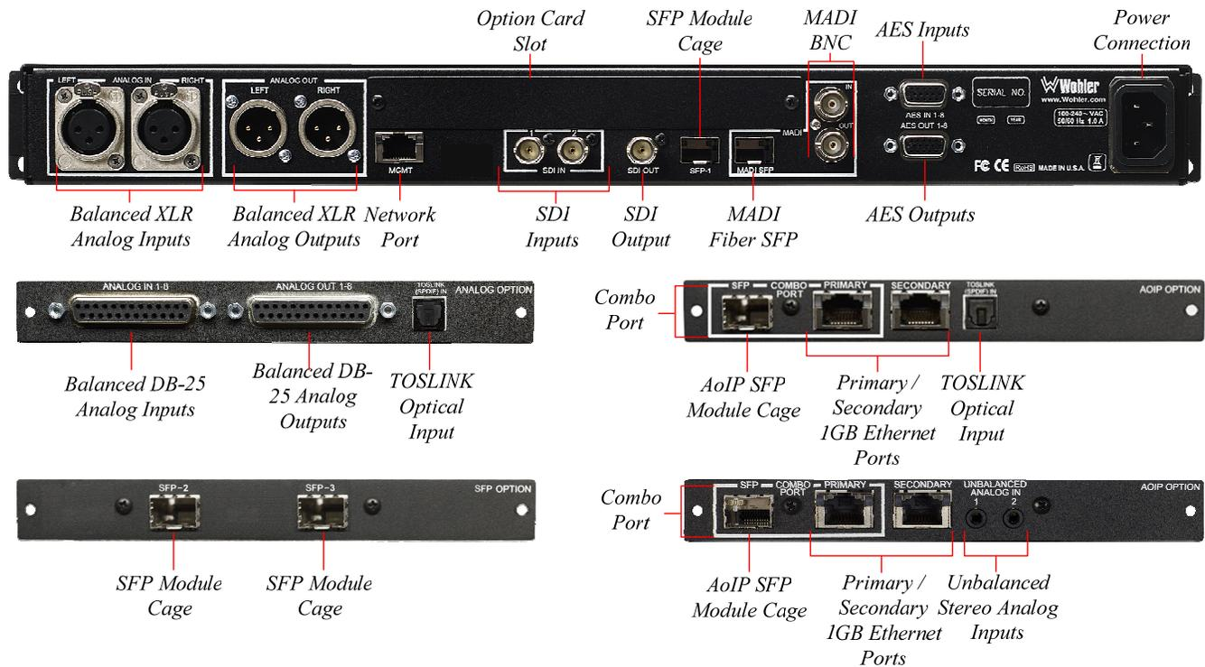
**Power Connection:** The *iAM1-MIX8* receives power from an AC inlet, which is a standard IEC receptacle for 100 to 240 VAC  $\pm 10\%$ , 50/60 Hz power connection. Four regional AC power cords, supplied according to shipping region, are available.
