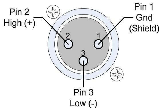
10. **Analog Outputs:** These male XLR connectors provide two balanced analog outputs: Left and Right. The source of these signals is the mix of audio as monitored by the internal speakers and is adjusted by the **Volume** control. The **Analog Outputs** are standard on the *iAM1-MIX8*. Refer to Figure 2-5 for the pinout of this connector.
