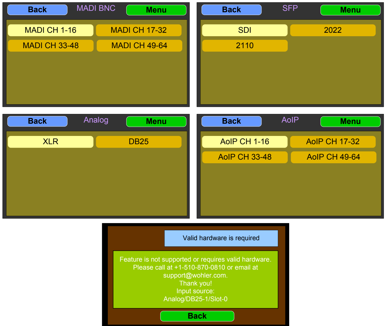
Figure 2-23: MADI, SFP, Analog, & AoIP Selection Screens:
